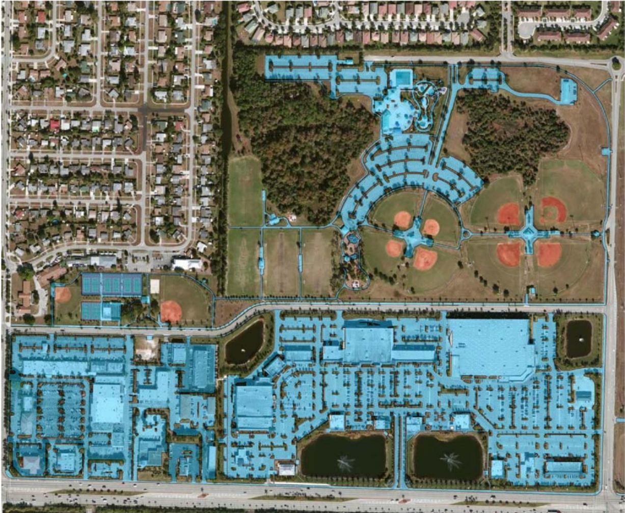
Figure 2-1 Nonresidential/Commercial Impervious Area Example
